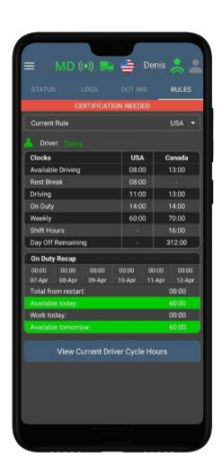
This page allows the driver to check the remaining hours. Same as HOS Calculator on the Hours of Service screen.
