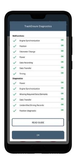
Malfunctions and Data Diagnostics indicate data inconsistency, failures or issues related to ELD. They can occur due to hardware or software failures, as well as external factors such as power failures, electromagnetic interference or physical damage to the device.
